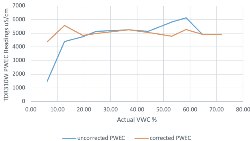
Figure 3. Uncalibrated and Calibrated PWEC Readings for the TDR310W in Cloud 50/50. The EC of the water used to flood the bag was 5000 uS/cm..
