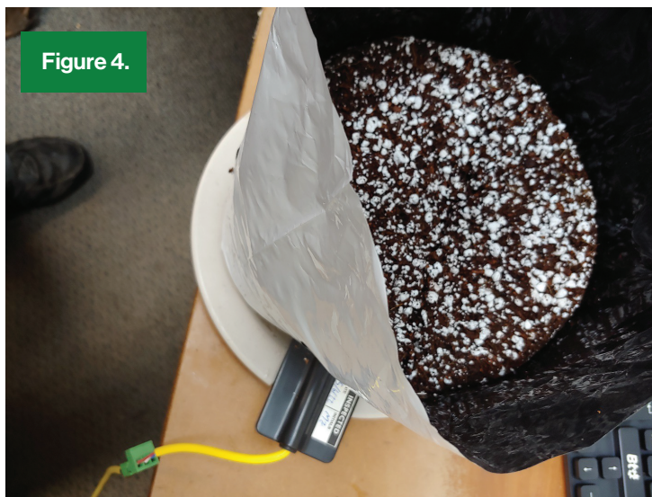
Figure 4. Cloud 50/50 material packed in a bag and wetted from the top using a sprinkler..
