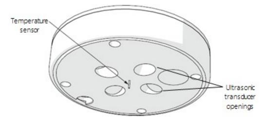
FIGURE 9-1. Temperature sensor and ultrasonic transducer openings
