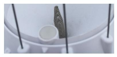
FIGURE 8-3. Correct installation: sensor is centered at the triangle
