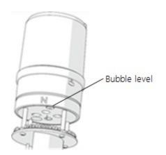
FIGURE 7-4. Bubble level on the ClimaVUE 50
