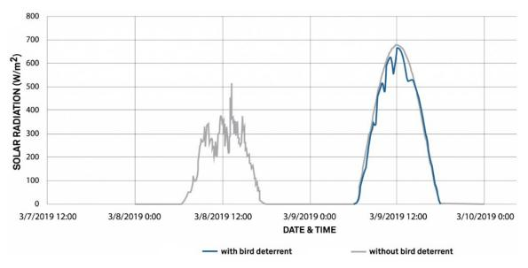
FIGURE 8-1. ClimaVUE 50 solar radiation data with and without bird spike kit
